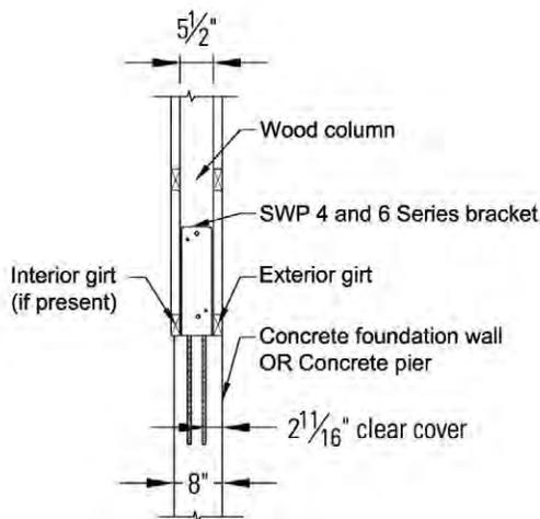
**Figure 12.1: Recommended Installation For SWP 4 and 6 Series Brackets**
