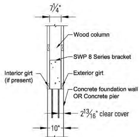
**Figure 12.2: Recommended Installation For SWP 8 Series Brackets**
